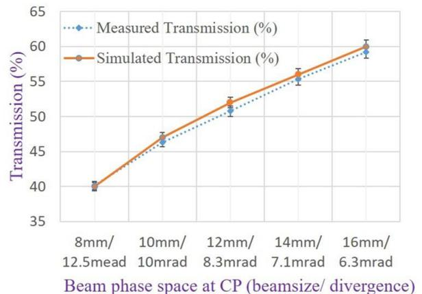
Figure 2: Beam transmission through gantry (simulation and measured) for transporting  $100 \pi \cdot \text{mm} \cdot \text{mrad}$  through gantry with different beam parameters at the CP [9].
