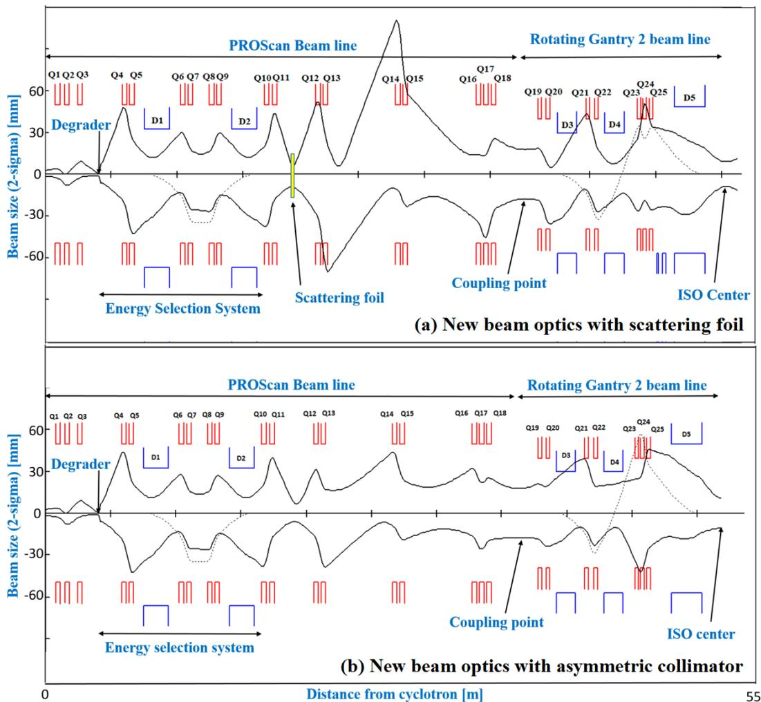
Figure 3: (a) shows the new beam optics with scattering foil transporting  $67 \text{ mm} \cdot \text{mrad}$  in X-plane and  $139 \pi \text{ mm} \cdot \text{mrad}$  in Y-plane up to scattering foil location and transporting almost  $145 \pi \text{ mm} \cdot \text{mrad}$  (in both planes) from scattering foil to isocenter. (b) shows the new beam optics with two asymmetric phase space selection collimators transporting  $100 \pi \text{ mm} \cdot \text{mrad}$  in both planes. [5,10]
