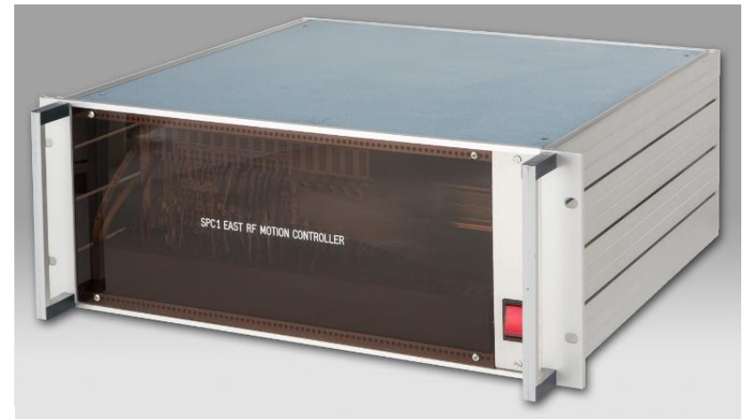
Power amplifier, anode, grid, trimmer, coupling capacitor and short circuit plate control
