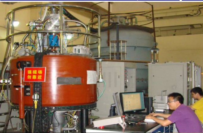
First, Second Small Cyc PET Cyclotron, 14 MeV, 450 \mu A
