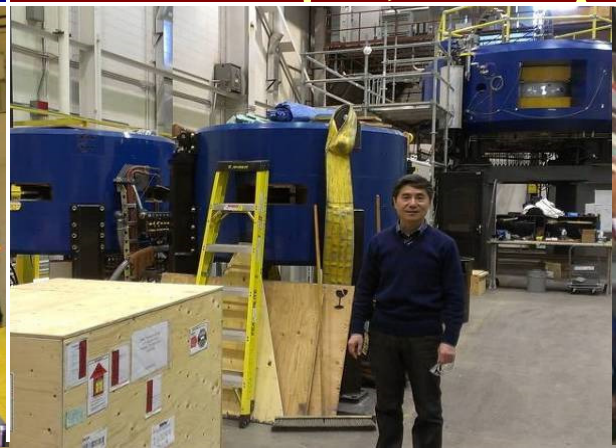
10 th Small Cyc, under construction for BNCT 3 rd to 9 th Small Cyclotron, 14 MeV, 100 \mu A to 400 \mu A, main parts for overseas
