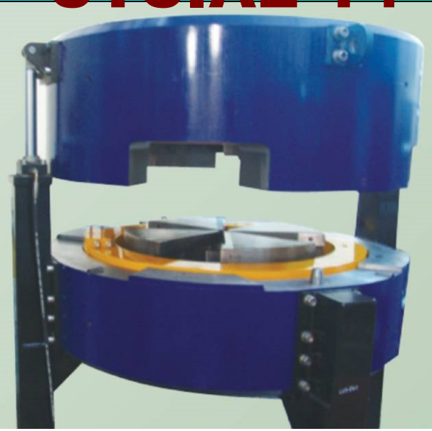
10 th Small Cyc, under construction for BNCT 3 rd to 9 th Small Cyclotron, 14 MeV, 100 \mu A to 400 \mu A, main parts for overseas
