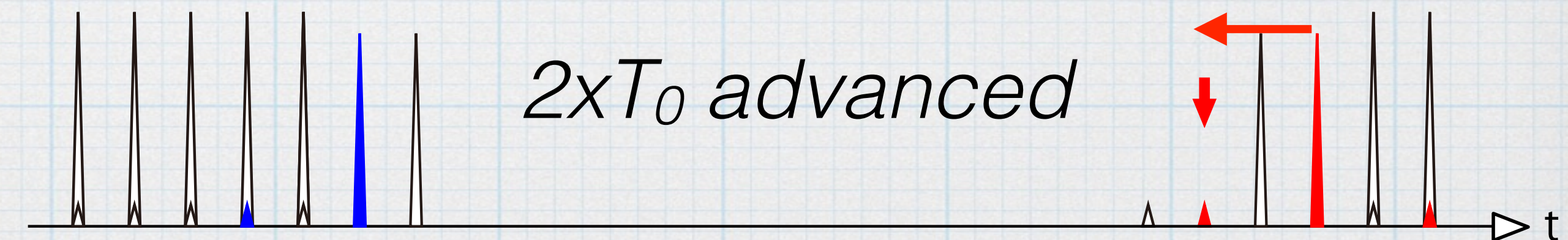
c) Extracted beams partly advanced by 1 turn
