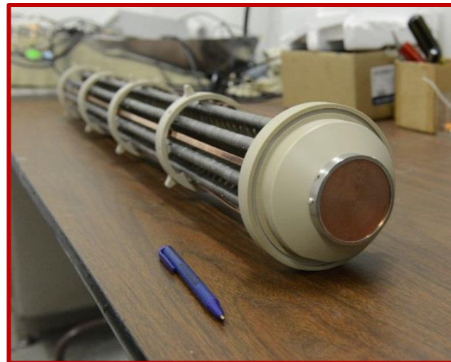
At either end: Mini-surfing carpets for differential pumping
