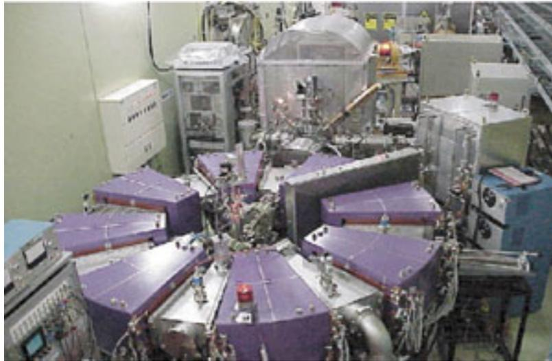
Proof of Principle machine finished in 1999 at KEK, demonstrated 1kHz rep. rate
