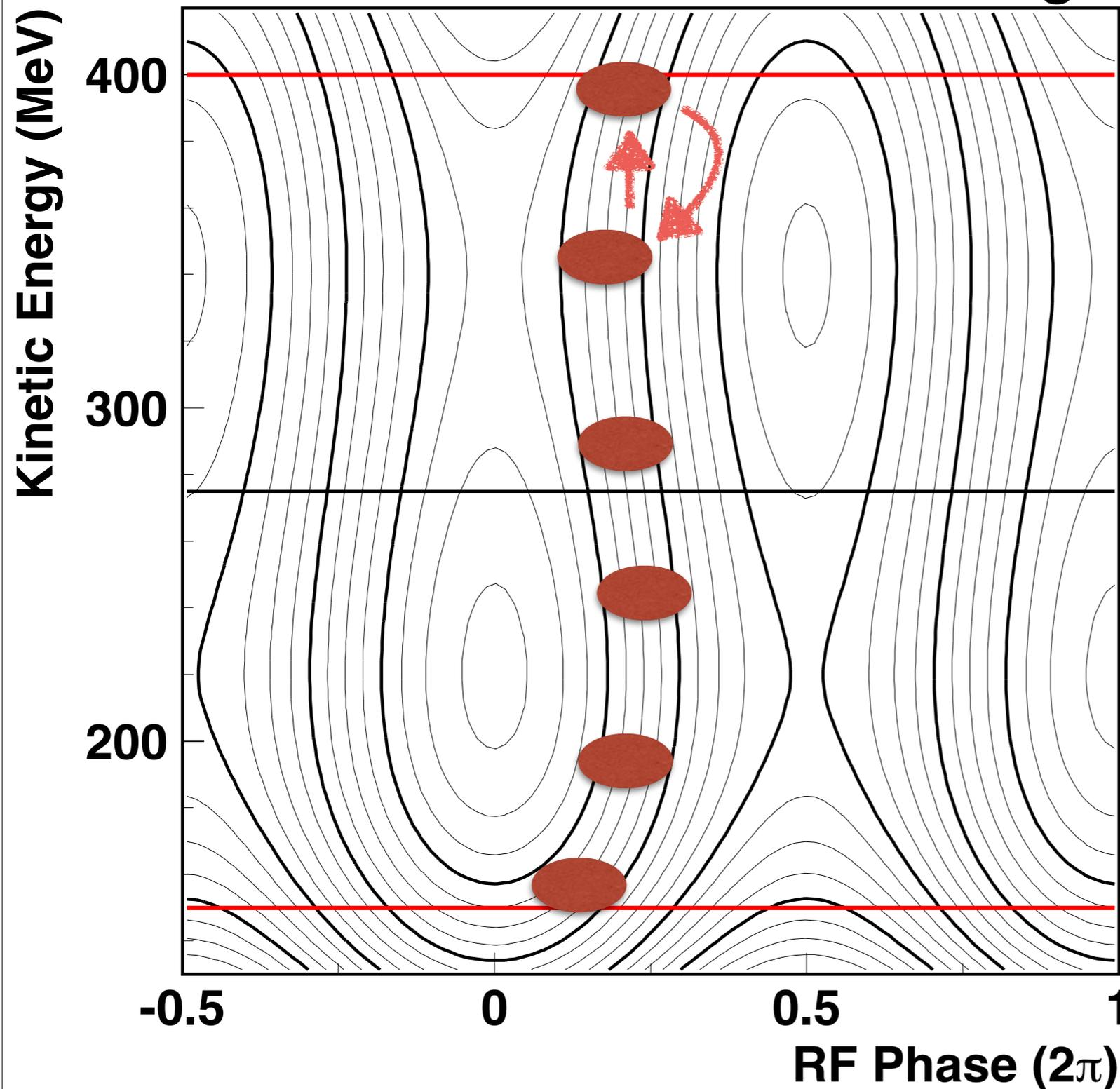
In the ordinary ERIT system, the ring is operated in a storage mode. However, in the extended ERIT system, the ring is in an acceleration mode. In this operation mode, since the beam hits the target at the maximum energy, the production efficiency of the secondary particles becomes high compared with the case of the storage mode.
