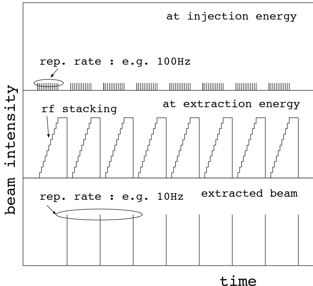
FFAG rings can provide long interval pulse for users, while the machine operation itself is kept at high repetition rate by using rf stacking after acceleration[1].
