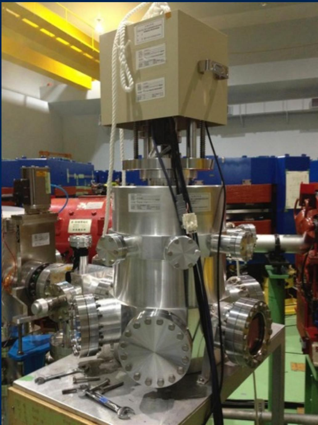
The irradiation port connected to the 150 MeV proton beam line. It has cryogenics and traction control machine inside which realize measurements under irradiation of the proton beam.
