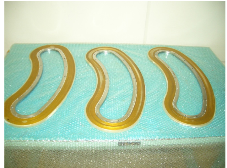
Each DP was impregnated with epoxy resin in vacuum.
