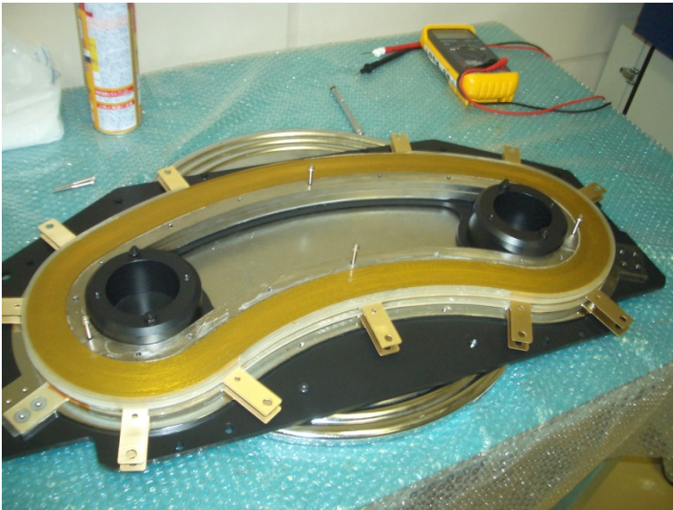
Three DP and cooling plates are stacked and impregnated with epoxy resin in vacuum.
