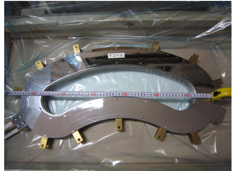
9 mm and 4.5 mm thick iron plates were put on outside and inside of coil, respectively.
