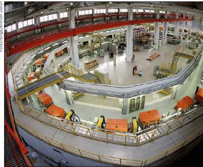
The COSY storage ring at the Forschungszentrum Jülich in Germany is being modified to search for very small electric dipole moments.
