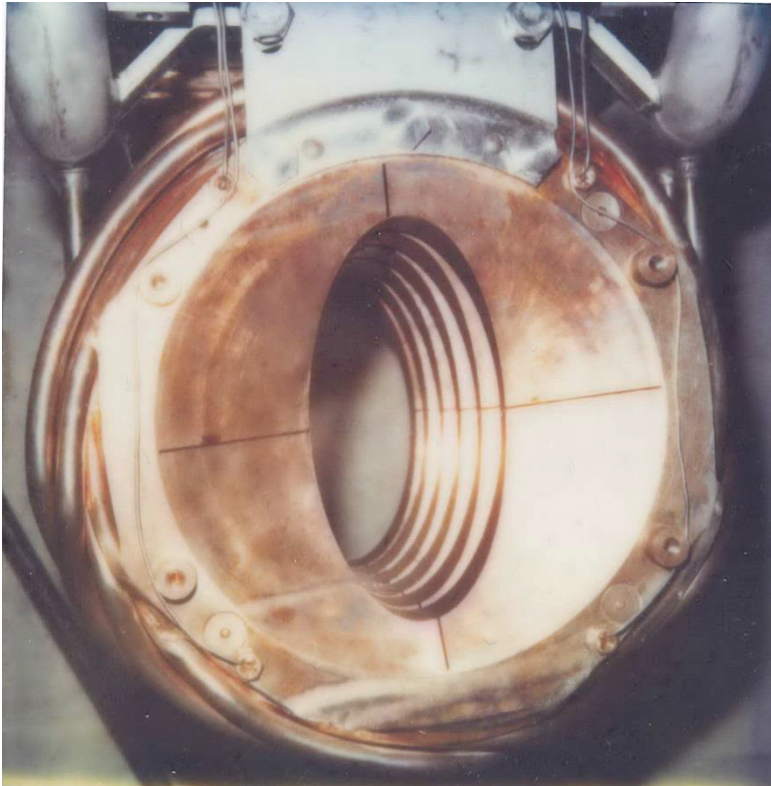
6 sections, cooling pipes
