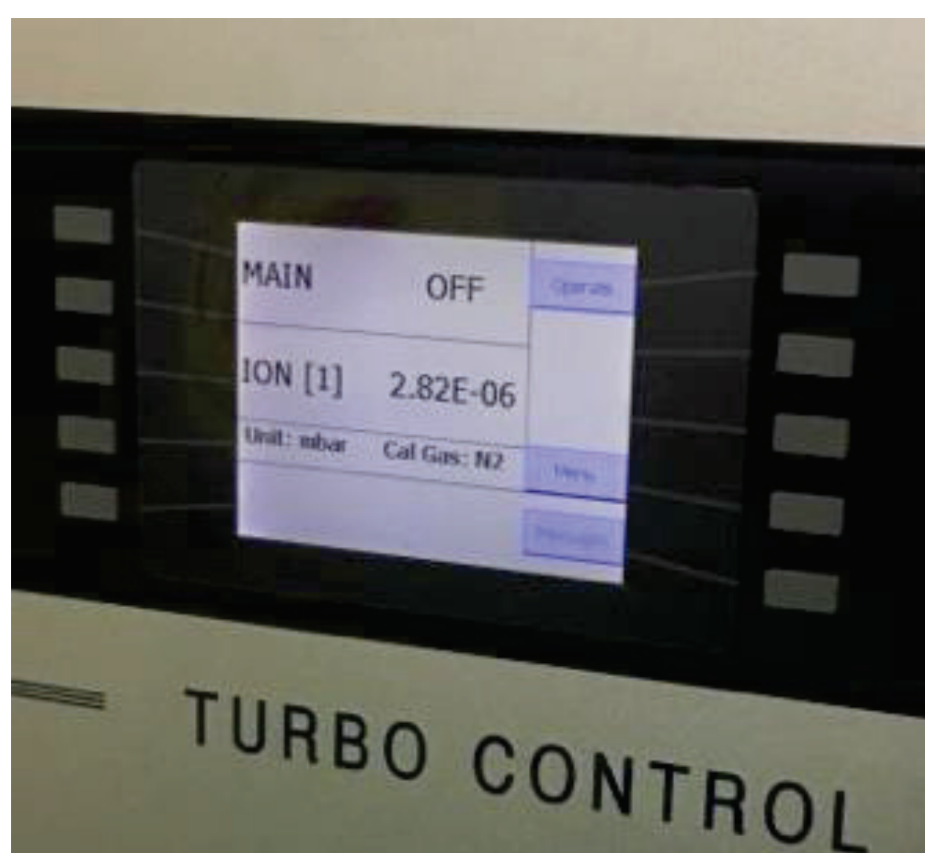
Figure 1 Vacuum level in ion source chamber with 8 SCCM gas injection
