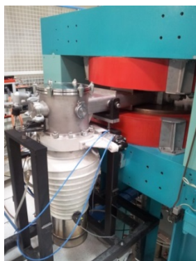
Figure 1: 1.7T test magnet and the vacuum system at AIMA.
