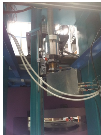
Figure 2: CYCLONE® 230 source arm mounted on a dedicated insertion system underneath test magnet.
