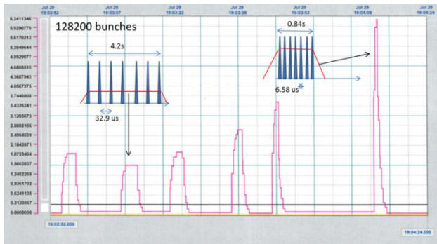
Figure 5: Intensity at the end of the beamline for the “start-stop” pulsation system.
