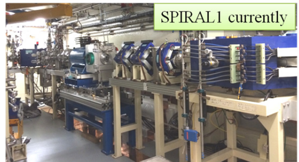
Figure7: Evolution of SPIRAL1 low energy p branch with the insertion of the charge booster.
