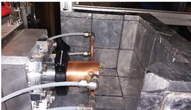
Figure 5: The FCs are shielded with 50 mm Pb bricks, to allow maintenance. Here only partial shielding is shown.
