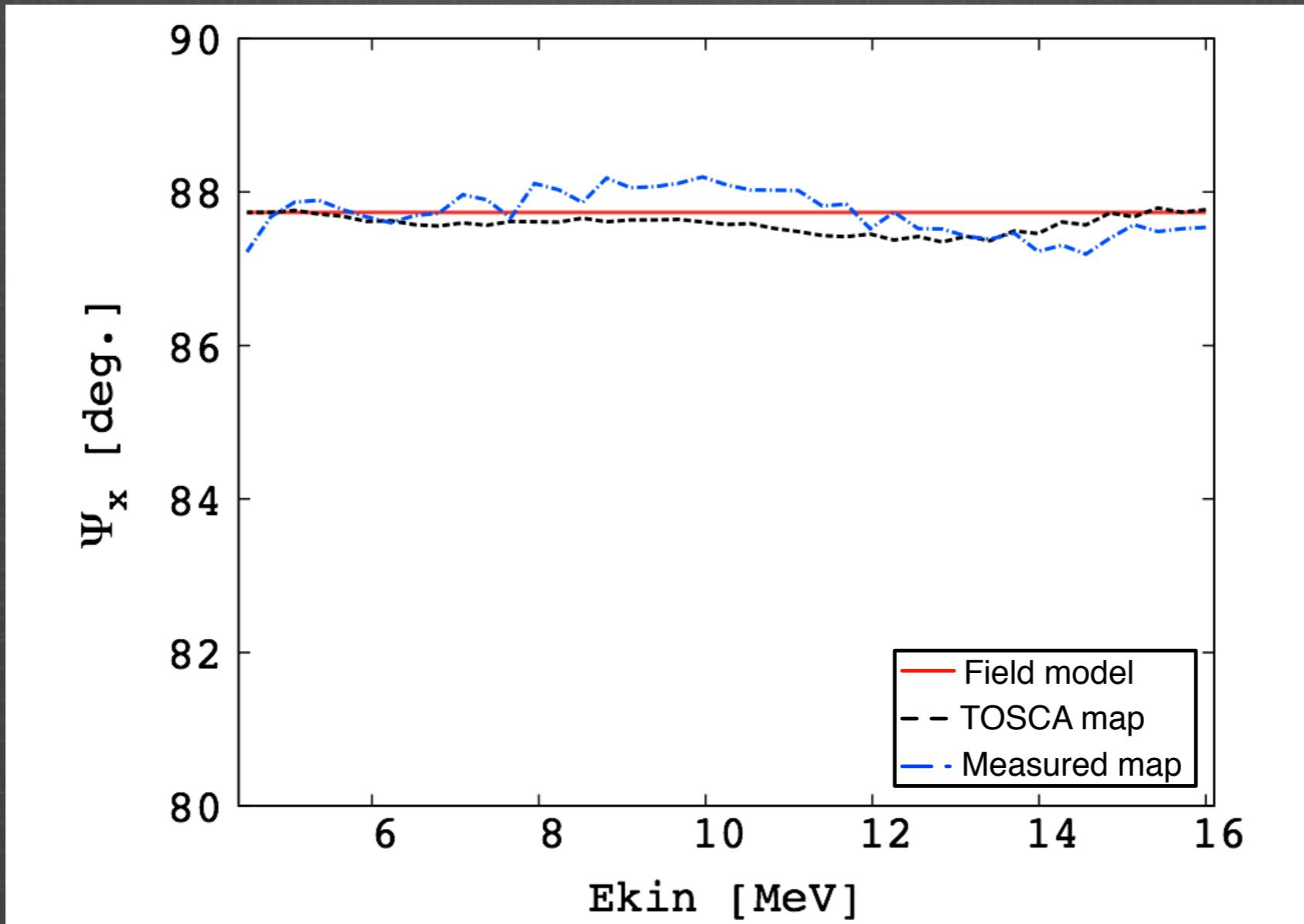
Horizontal phase advances vs kinetic energy with field model (plain red), in TOSCA field map (black dashed) and in measured field map (mixed blue).
