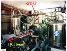
Figure 2: SERSE source installed to injector beam line.
