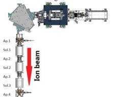
Figure 5: SuSI ion source and the collimation line.
