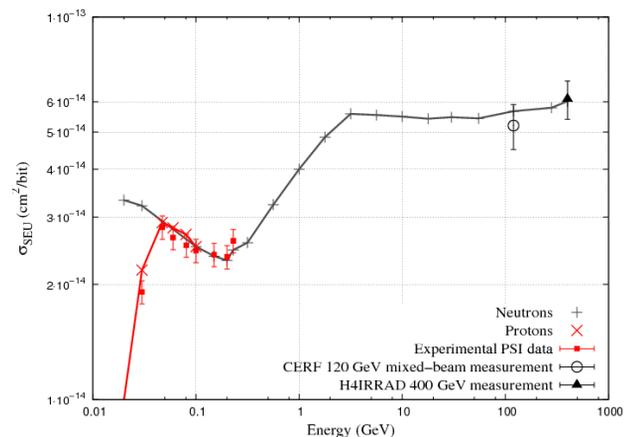
Figure 2: SEU cross section of the ESA SEU monitor.
