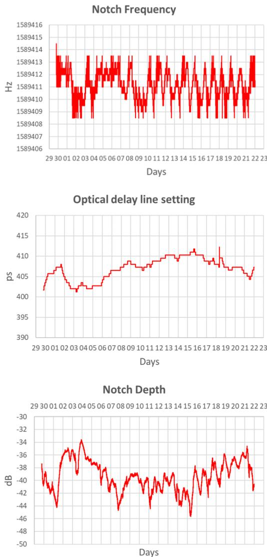
Figure 3: Notch frequency at 1000<sup>th</sup> harmonic, notch depth and programmed delay to keep stability over a period of ~four weeks from 29.09.2021 to 23.10.2021.
