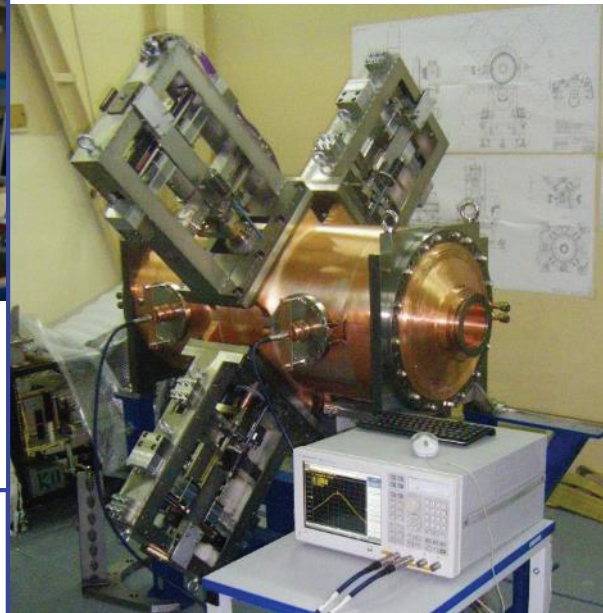
f_0 = 11.1 \div 13.6 \text{ MHz} Q_0 = 3\,600 (@ 12.2 MHz) Ready for high power tests.
