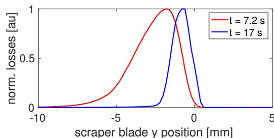
Figure 4: Normalised beam losses as a function of the vertical scraper position before (red) and after (blue) cooling. The width of the signal corresponds to half the beam size.
