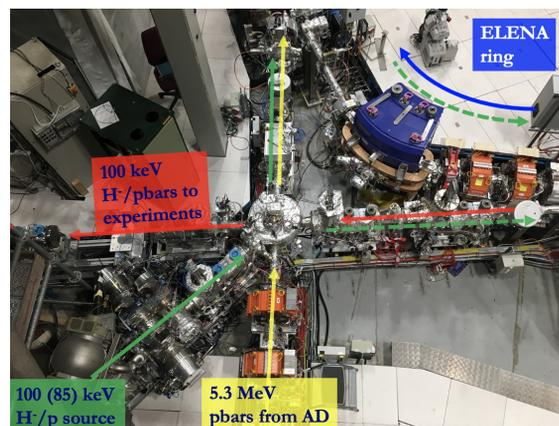
Figure 2: Injection and extraction lines toward main experiments. The ion source is partially visible in the bottom left corner. The possible beam paths are highlighted.
