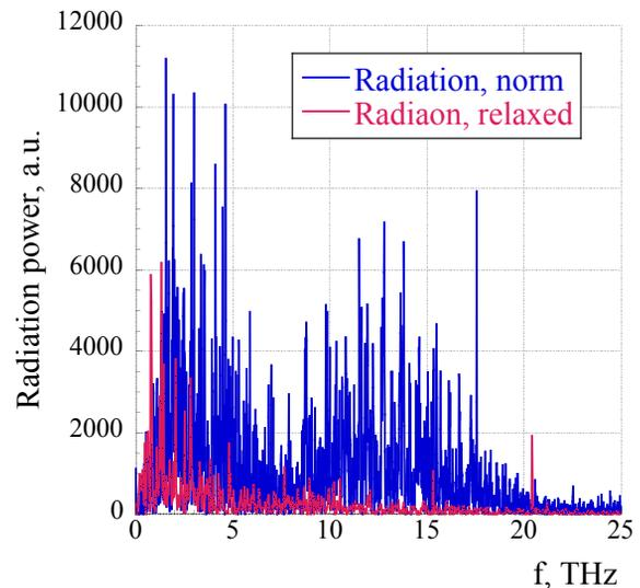
Figure 4: Radiation spectrum of the compressed 0.7 nC electron bunch profile at the exit of the SRF linac simulated by Impact-T. Blue colour line is for strong focusing lattice (used during RHIC Run 18) and Red colour lines are for a relaxed lattice of the CeC accelerator. Horizontal axis is the frequency measured in THz.
