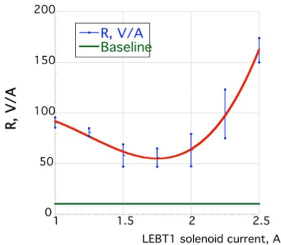
Figure 8: Redline is the measured ratio of the lock-in amplifier voltage to the average beam current,  $R$ , as function of the current in LEBT1 solenoid. Green line shows the baseline for  $R$  value corresponding to the shot noise.
