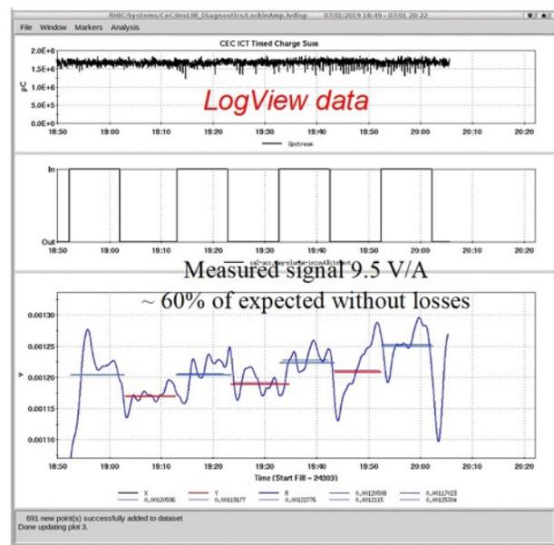
Figure 7: Illustration of the evolution of signal from lock-in amplifier and the need for the MDM method. Top graph shows the charge per bunch train. The middle graph shows location of the reflecting mirror (IN/OUT). The bottom graph shows evolution of the lock-in signal with time constant of 30 seconds. Significant drifts illustrate the need for averaging and the MDM method for accurate measuring the radiation power at this level.
