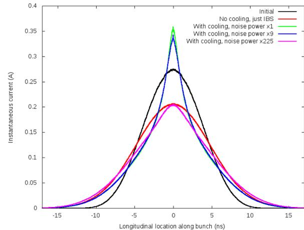
Figure 10: Evolution of the 26.5 GeV/u ion bunch profile in RHIC. Black - initial profiles at  $t=0$ . All other profiles are shown at  $t=40$  minutes. Red— evolution of witness bunch without cooling; green – cooled with e-beam having natural shot noise; blue- cooled with e-beam with 9 time increase in the noise power; crimson - e-beam with 255 time increase in noise power.
