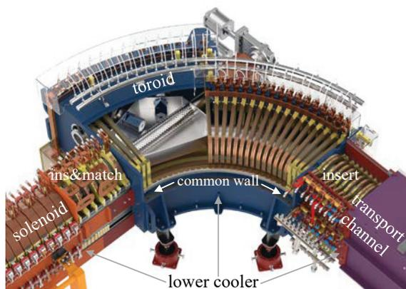
Figure 7: Layout of segment C–T–S.
