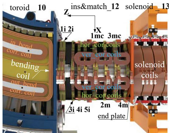
Figure 9: Magnetic elements of units 10, 12 and 13.
