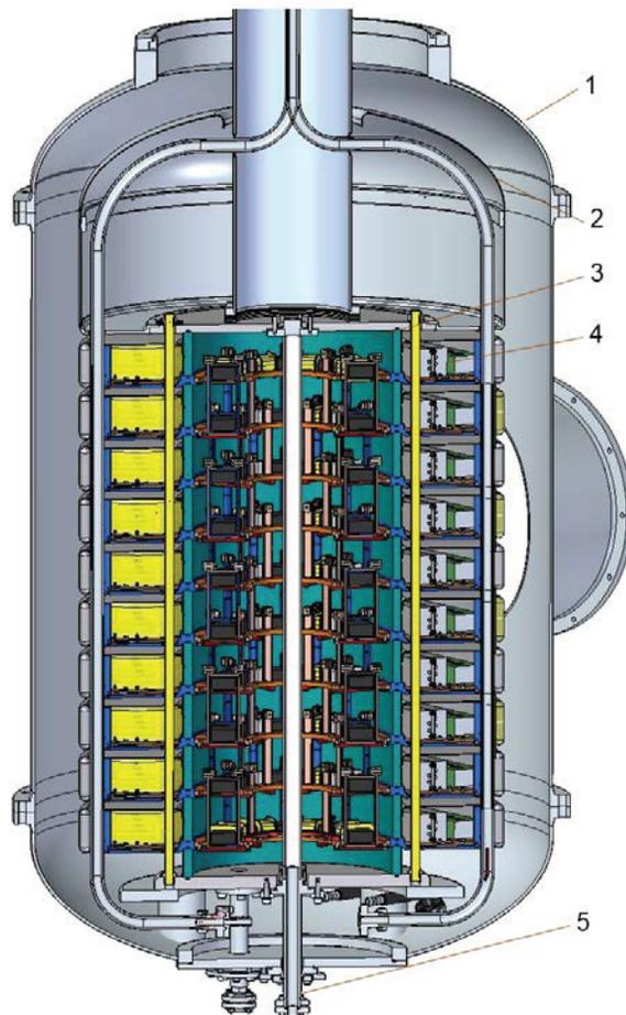
Figure 1: The structure of the high voltage column. 1 – SF<sub>6</sub> tank; 2 – shielding cover; 3 – high voltage cascade transformer; 4 – high voltage section; 5 – isolating and cooling oil tubes.
