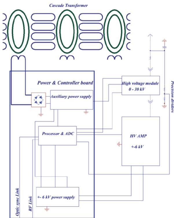
Figure 4: The structure of the high voltage section.
