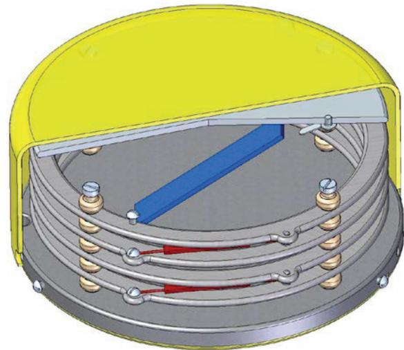
Figure 3: General view of the precision high voltage divider.
