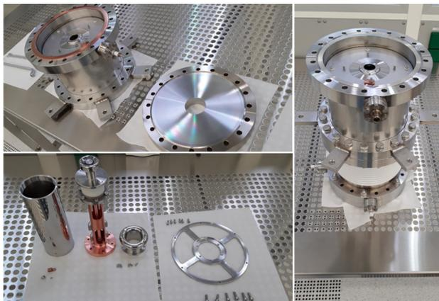
Figure 9: Different stages of assembly of the redesigned source in the HIM cleanroom.
