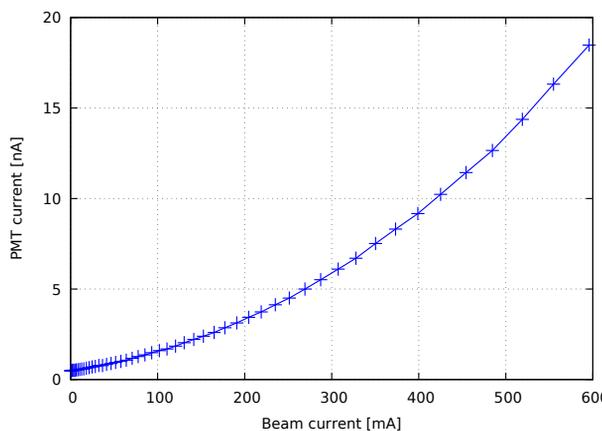
Figure 6: Photon signal for fixed lens and slit positions at different beam currents.
