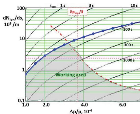
Figure 7: Estimates of critical parameters of the ion beam in NICA Collider at ion stacking.
