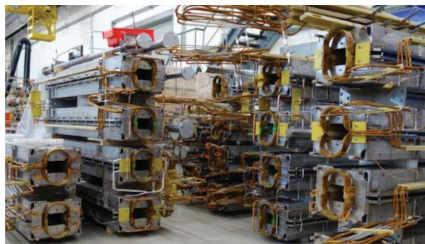
Figure 4: SC “twin” dipoles of Collider.
