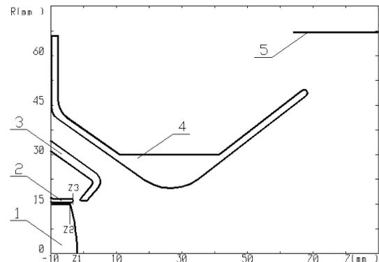
Figure 1: Geometry of electrodes of the electron gun with variable beam profile.
