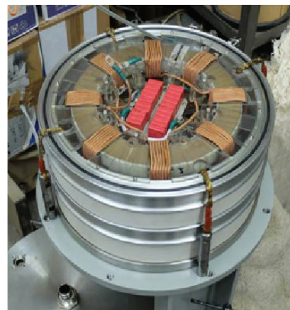
Figure 8: Cascade transformer on test bench for solenoid component after tilting individual coils of solenoid by 4 mm.
