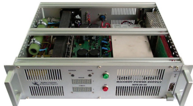
Figure 3: Power supply MPS-20-50.
