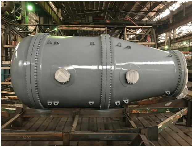
Figure 9: Vessel for high voltage equipment produced in Novosibirsk
