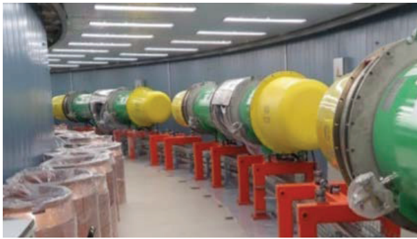
Figure 2: SC magnets of the Booster in the yoke of the dis-mounted Synchrotron.
