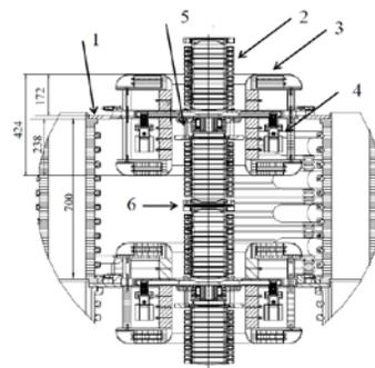
Figure 3b: Arrangement of two solenoids on different decks with 600kV acceleration in between [6]. 1: main construction frame, 2: acceleration tube 3: solenoids 4: vacuum pumps, 5 bellows and beam position monitor, 6: flange connection.
