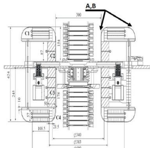
Figure 3a: Mounting of a solenoid on the module baseplate around the acceleration tube [6]. Dimensions in mm. Points A and B are regions of high field strength.
