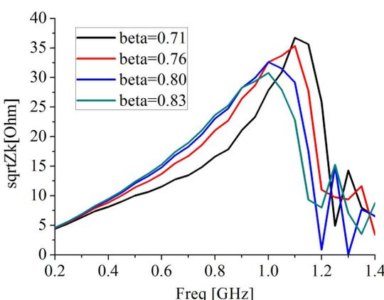
Figure 13: kicker longitudinal shunt impedance of Faltn type with 0.75 m, when rectangular aperture is 200\*120 mm.
