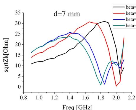
Figure 9: kicker longitudinal shunt impedance of Faltn type ,when the distance from electrode to slot is 7 mm.
