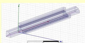
Figure 8: A quarter HFSS simulation model with circular aperture Ø=118 mm, slot section=0.75m.
