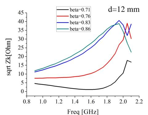
Figure 11: kicker longitudinal shunt impedance of Faltn type ,when the distance from electrode to slot is 12 mm.
