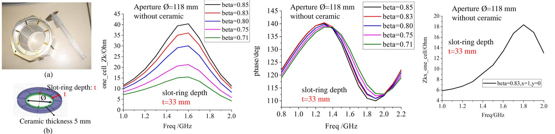
Figure 1: (a) : 8 slot-rings prototype from FZJ; (b): one slot-ring HFSS model with 8 electrodes , cell length=13.5 mm.
