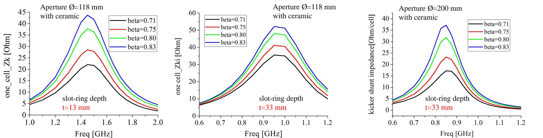
Figure 5: Slot-ring kicker longitudinal shunt impedance per cell with ceramic Ø=118 mm when cell length is 13.5 mm.
