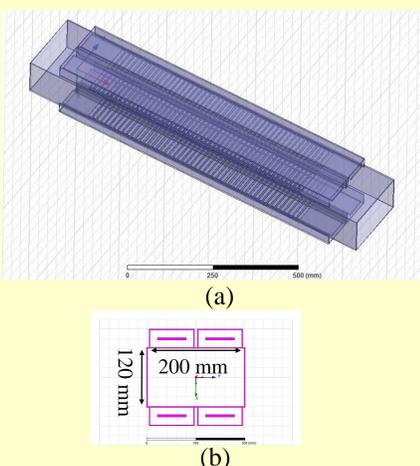
Figure 12 (a): A full HFSS simulation model with rectangular aperture 200\*120 mm, slot section=0.75 m; (b): cross section.
