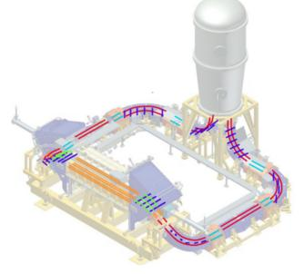
Figure 1: Image of the 2 MeV electron cooler. Equally colored symbolic field lines represent coils that share the same power supply. Orange: "Cooling section", red: "Longitudinal field", blue: "Bending field", green: "Toroid 45° field", and cyan: "Straight field".
