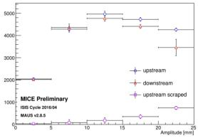
Figure 9: A comparison between the upstream and downstream amplitude distributions for the 3 mm nominal beam and the 6 mm nominal beam. The particles that were reconstructed upstream but were scraped before reaching the downstream tracker are also shown.
