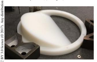
Figure 4: Polyethylene wedge piece machined for use in the MICE experiment. Wedge for mu2e would have similar dimensions. (Inner radius is ~20cm).
