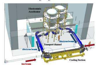
Figure 1: 3D design of 2 MeV COSY cooler.
