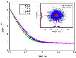
Figure 6: Cooling process with long pulse width of e-beam and the particle distribution before and after cooling.
