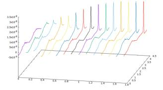
Figure 7: The ion bunch was cooled by pulsed electron beam. There are two ion bunches in the ring but only one was cooled by pulsed electron beam.
