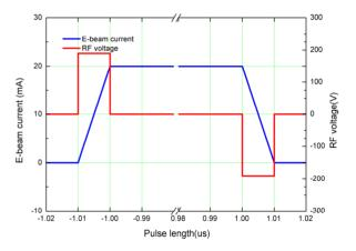
Figure 4: RF bucket with amplitude of 150V can be created by an electron pulse, the peak current is 50mA and the rise/fall time is 10ns.
