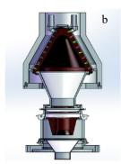
Figure 2: Structures of the electron gun and collector for cooler of HIAF.
