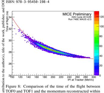
Figure 8: Comparison of the time of the flight between TOF0 and TOF1 and the momentum reconstructed within the upstream tracker. The red dashed line describes the theoretical results for a particle with the muon mass.
