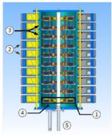
Figure 6: Design of high-voltage system. 1 - section transformer, 2 - electronic section, 3 - section transformer metal ring and ceramics, 4 - vessel filled by oil, input and output of oil.
