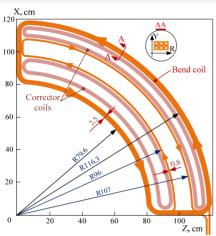
Figure 2: Design of bending magnets.
