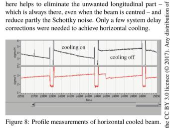
Figure 8: Profile measurements of horizontal cooled beam.
