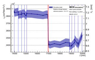
Figure 9: 9 %-contour volume evolution through the MICE cooling channel.
