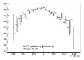
Figure 6: Figures showing the downstream tracker acceptance in  $\theta_X$  (top) and  $\theta_Y$  (bottom).
