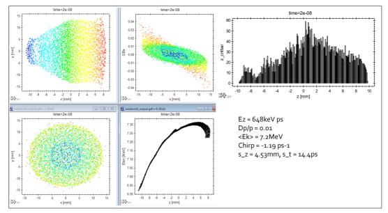
Figure 5: Particle distributions at the end of the booster for the injector. Each slice of the distribution has good magnetization but the slices do not have the same Twiss parameters so the projected emittance is larger than the specification.
