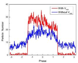
Figure 2: Final beam distribution after cooling with Vkick and without Vkick.
