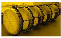
Figure 5: Photograph of a scintillating fibre tracker under construction. The yellow light was required in order to prevent damage the fibres.
