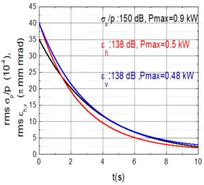
Figure 10: Evolution of rms parameters of the antiproton beam for simultaneous cooling in all 3 planes. P<sub>max</sub> is the initial cw power at the kicker within the 1-2 GHz band. Four times this value (i.e. to account for statistical beam signal fluctuations) is just within the installed microwave power of 8 kW (power amplifiers at kickers).
