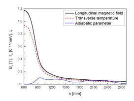
Figure 4: Variation of Longitudinal magnetic field  $B_s$ , transverse electron temperature  $T_{tr}$ , and adiabatic parameter  $\xi$  along the longitudinal coordinate s.
