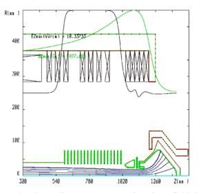
Figure 8: The collector structure of SRing, field in collector region, and beam profile in collector.
