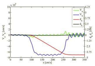
Figure 10: Variation of transverse velocity and electron displacements in two directions (without deflector).
