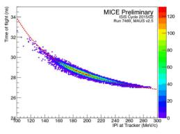
Figure 9: Time-of-flight distribution between TOF0 and TOF1 as a function of the total momentum measured in the upstream Tracker. The absence of other populations indicates selection of a pure muon sample.
