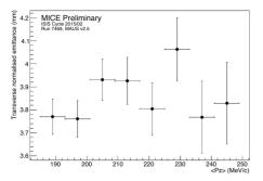
Figure 10: Transverse normalised emittance of 8 MeV/c longitudinal momentum bins.
