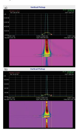
Figure 6: Longitudinal cooling of  $7*10^9$  (a) and  $2*10^8$  particles (b).
