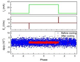
Figure 1: The distribution electron beam current and its electric potential at the edge, and distribution of particles in phase space when pulse e-beam is applied.
