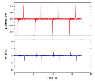
Figure 5: The BPM signal was observed clearly, even without RF system. The width is the same as electron pulse.
