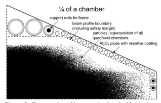
Figure 7: Topography of beam and tubes inside the hexagonal quadrupole/sextupole chamber.
