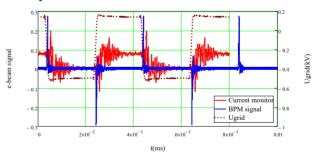
Figure 1: Modulated voltage on the grid electrode of the gun (dash line), pulsed electron beam current (red) and BPM signal generated by pulsed electron beam in the cooler.
