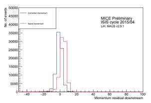
Figure 5: Figures showing the residual between the momentum before and after correction up- (top) and downstream (bottom) and the momentum determined from MC truth.
