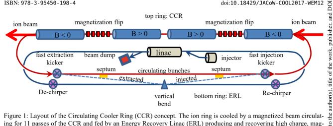
Figure 1: Layout of the Circulating Cooler Ring (CCR) concept. The ion ring is cooled by a magnetized beam circulating for 11 passes of the CCR and fed by an Energy Recovery Linac (ERL) producing and recovering high charge, magnetized bunches at a 43.3 MHz repetition rate.
