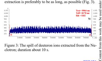
Figure 3: The spill of deuteron ions extracted from the Nuclotron; duration about 10 s.
