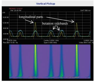
Figure 11: Difference signal of vertical plane.
