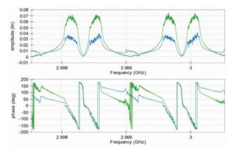
Figure 7: First transverse open loop measurement with and without notch-filter.
