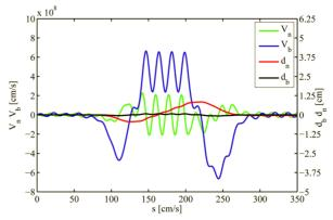
Figure 11: Variation of transverse velocity and electron displacements in two directions (with a deflector).
