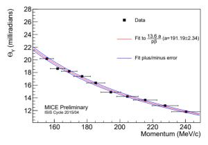
Figure 8: The results of the scattering analysis using data from all three nominal beam settings. Scattering widths are reported after application of deconvolution.
