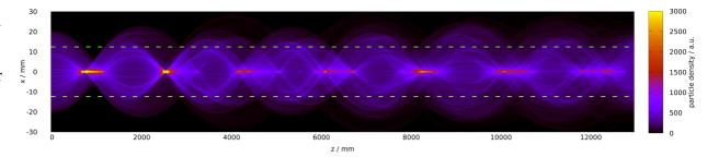
Figure 3: Particle density development for  $r_e < r_p$  of an initially homogeneous proton beam (I = 5 mA, E = 50 keV) which interacts with an ideal static electron column (edge with green dashed line) with a density ratio of  $n_e = 12n_p$ .
