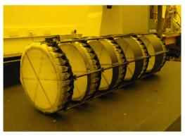
Figure 7: The MICE Tracker detectors showing the 5 stations each consisting of three planes of WLS fibres.
