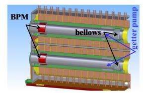
Figure 5: Design of the cooling section.
