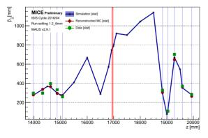
Figure 3: Beta function profile in the MC truth (blue line), reconstructed MC (red circles) and data (green squares).
