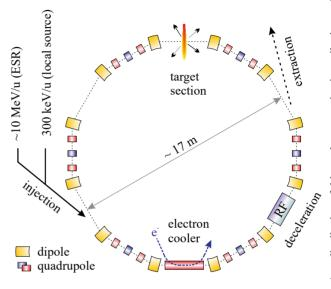
Figure 1: Schematic layout of CRYRING@ESR. The main components; injection, extraction, electron cooler, RF section, and the target section are indicated.
