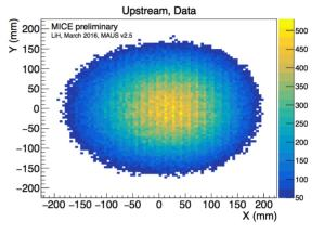
Figure 2: Upstream position distributions for a 200 MeV/c muon beam in the LiH data after particle selection.
