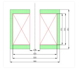
Figure 2: Cross section of the gun solenoid.
