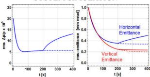
Figure 9: Momentum spread, horizontal and vertical emittance during 3D-cooling for 200 s, and beam blow-up when cooling is turned off.
