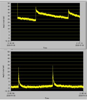
Figure 2: The DCCT signals of stored beam without (above) and with (below) pulsed electron beam.
