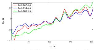
Figure 2: Vertical field component measured at different value of the longitudinal field. Red -1~kG, blue -800~G, green -700~G.
