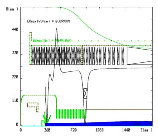
Figure 5: The geometry of the magnetic system for guns of SRing.
