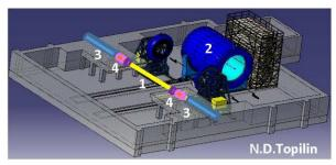
Figure 7: The MPD before final assembling: 1 - beam pipe 2 - solenoid, 3 - final focus lenses, 4 - FFD and FHC for Collider luminosity tuning.
