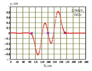
Figure 4: Oscillation of orbit in the bending magnet.
