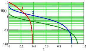
Figure 4: Dependence of  $\delta(t)$  on time at constant particle flux  $J(\delta)$  (arb. units) at slow resonant extraction of Gaussian beam of different values of the beam transverse  $(\sigma_x)$ and longitudinal ( $\sigma_p$ ) emittances:
