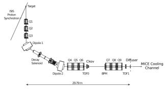
Figure 4: Layout of the transfer line from the ISIS synchrotron through to the MICE Cooling Channel.
