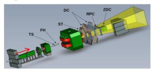
used under the terms of the CC BY Figure 5: Scheme of the BM@N detector: TS - Target Station, FH – Forward Hodoscopes, ST – Straw tube Tracker, <sup>2</sup> DC – Drift Chambers, RPC – Resistive Plate Chamber, ZDC - Zero Degree Calorimeter; arrow indicates the direction of the primary ion beam.
