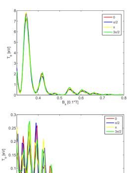
Figure 3: Dependence of transverse electron temperature upon the longitudinal magnetic field strength after toroid with (upper) and without (lower) the bending electro-static field. Electrons start from different initial phase advance of  $0, \pi/2, \pi, 3\pi/2$  in Larmor procession.
