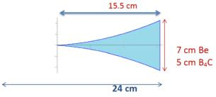
Figure 5: Cross-section of a wedge to be inserted at the high dispersion point of the mu2e transport solenoid. The wedge is offset from the center line by  $\sim$ 8.5cm so that low-energy  $\mu$ 's pass without touching the wedge; higher-momentum  $\mu$ 's lose energy toward  $P_{\mu} \sim$ 40 MeV/c.
