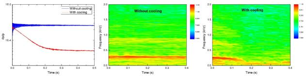
Figure 5: Beam spectrum in frequency domain for pulse e-beam cooling. The initial momentum spread and pulse width are 2E-4 and 600 ns respectively. The sidebands is caused by the oscillation within pulse electron beam.
