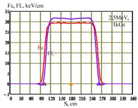
Figure 3: Centrifugal and Lorentz forces in 90 bend magnets
