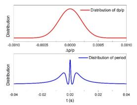
Figure 4: The distribution of momentum spread and period time for ion beam.
