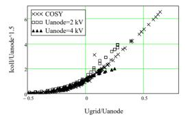
Figure 7: Volt-ampere characteristic of the gun at different setups of the cooler parameters.
