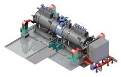
Figure 6: The MICE cooling channel showing the two spectrometer solenoids in grey and the absorber focus coil in blue.
