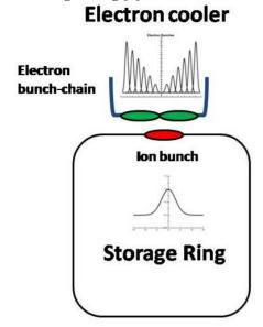
Figure 1: The longitudinal relation between the ion bunch in the storage ring and electron multi-bunch in the electron cooler.
