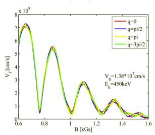
Figure 9: The dependencies of the velocity  $V_t$  on magnetic field.
