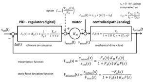
Figure 5: Stable adjustable control loop model with PID regulator and 2-pole path.
