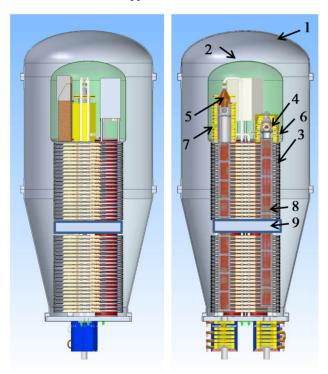
Figure 6: Design of the electrostatic accelerator of NICA cooler. High-pressure vessel for SF<sub>6</sub> is 1, high-voltage terminal (HVT) is 2, ihigh voltage section is 3, electron gun is 4, electron collector is 5, magnetic system of the electron gun is 6, magnetic system of the electron collector is 7, acceleration tube is 8, middle section is 9.
