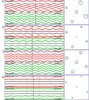
Figure 3: Trajectories in straight section. Red is projection in x, green is projection in y. First initial uncompensated beam, second larmor corrected, third galloping corrected, final larmor corrected again.
