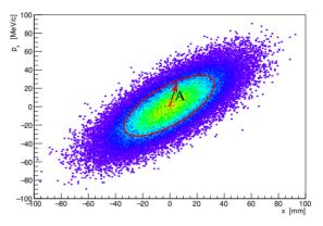
Figure 2: Example phase-space distribution with a contour of equal amplitude marked in red.
