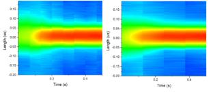
Figure 8: Preliminary data shows a difference of cooling process by different electron pulse width (2.5 µs left and 1.0 µs right).
