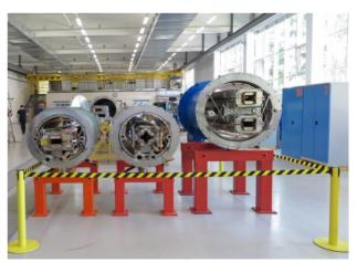
Figure 6: Serial dipole magnet and quadrupole lens doublet for Booster and preserial "twin" dipole magnet for Collider Full energy range two parts of energy range.
