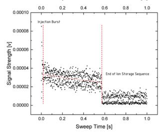
Figure 3: Storage time measurement using the Schottky noise signal. The moments in time when the ions are injected and dumped are marked with red dashed lines. The red line is an exponential fit to the data points that yields a storage time constant of 1.9(2) s.
