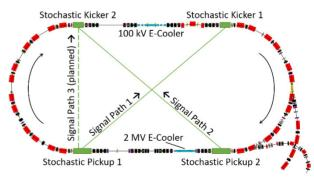
Figure 2: Cooling systems at COSY: Two electron coolers, the high energy SC system at signal path 1, the deprecated vertical and longitudinal system at path 2, and the planned low energy system at path 3.
