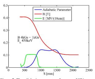
Figure 7: The adiabatic parameters for guns of SRing Figure 7 shows the adiabatic parameter of SRing. It can be found that the adiabatic parameters are << 1 for the 450keV electron beam.
