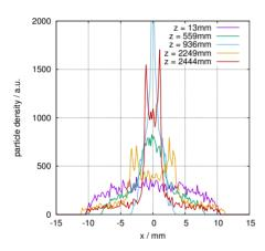
Figure 4: Beam profiles of a proton beam interacting with an ideal electron column for  $r_e < r_p$ .
