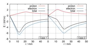
Figure 2: Radial electric fields of the initial homogeneous distributions for case 1 ( $r_e < r_p$ ) and case 2 ( $r_e > r_p$ ) split into the proton and electron part and the resulting field.
