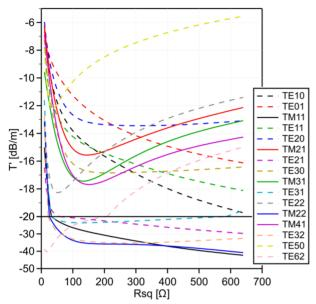
Figure 8: Dependence of damping on sheet resistance.
