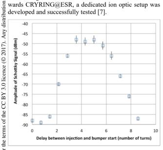
Figure 2: Present efficiency of the multiturn injection scheme. The amplitude of the Schottky noice signal is used as intensity monitor of the stored ion beam after injection at varying times after the bumper ramp start. This time is expressed in number of turns. One turn takes about 7 µs at injection energy.
