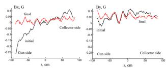
Figure 1: Horizontal (left) and vertical (right) magnetic field components before (black) and after (red) coils adjustment.
