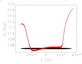
Figure 4: Longitudinal phase space after 20 passes with an RF cavity compensating the energy loss and chirp. The compensation is not perfect but it is possible to get close to the correlated energy variation specification in Table 1 of 6x10<sup>-4</sup> peak-to-peak.
