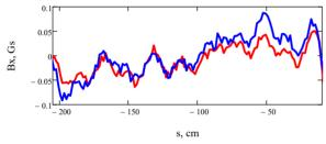
Figure 5: Horizontal field component before (red) and after (blue) all screws were tightened.
