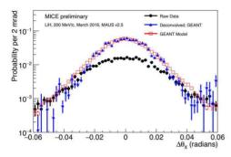
Figure 12: Projected (below) and 3D (above) scattering distributions of 200 MeV/c muons passing through the LiH absorber.
