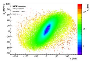
Figure 5: Scatter plot of the particles in the tracker station that is furthest downstream in the  $(x, p_x)$  projection. The color scale represents the individual particle amplitudes.
