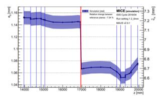
Figure 6: 9%-subemittance evolution through the MICE cooling channel.
