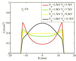
Figure 3: Electron beam current density distribution with different voltage on grid and anode.
