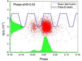
Figure 8: Beam distribution after cooling with the pulsed e-beam which have a phase shift (0.05) in longitudinal.
