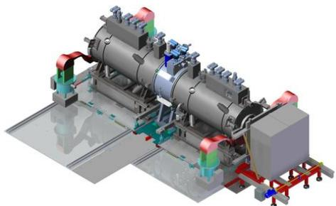
Figure 6: The MICE cooling channel showing the two spectrometer solenoids in grey and the absorber focus coil in blue.
