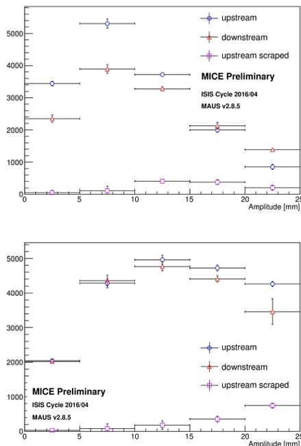
Figure 11: Change in amplitude distribution for the 3 mm 140 MeV configuration (above) and for the 6 mm 140 MeV configuration (below) are shown. Their transmission is  $\sim 90\%$  and  $80\%$  respectively. Blue circles show the amplitude of upstream events, red triangles show the amplitude of downstream events while magenta squares show the amplitude of upstream events that are not observed downstream.
