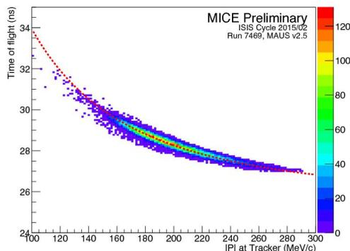
Figure 9: Time-of-flight distribution between TOF0 and TOF1 as a function of the total momentum measured in the upstream Tracker. The absence of other populations indicates selection of a pure muon sample.
