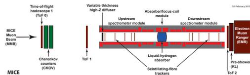
Figure 3: Schematic of the International Muon Ionization Cooling Experiment (MICE), with the beam entering from the left.
