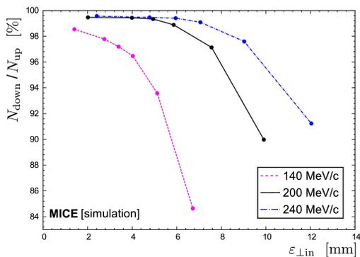
Figure 2: Change in transmission (in percent) vs. input emittance for a range of MICE beam momenta.
