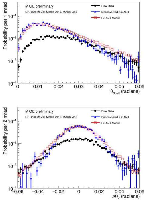
Figure 12: Projected (below) and 3D (above) scattering distributions of 200 MeV/c muons passing through the LiH absorber.
