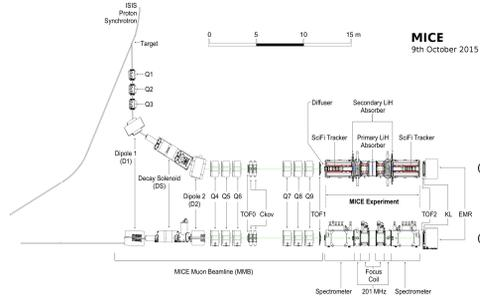
Figure 5: Schematic of the ISIS proton synchrotron and the MICE beam extraction magnets.
