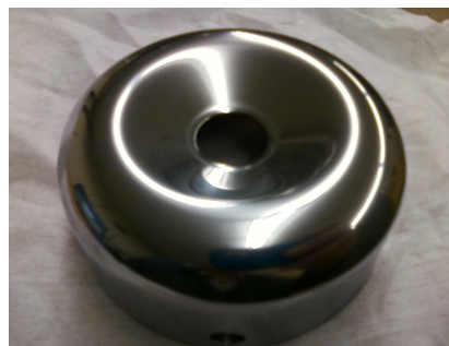
Diamond-paste polished Ti-alloy: a traditional “hard” electrode
