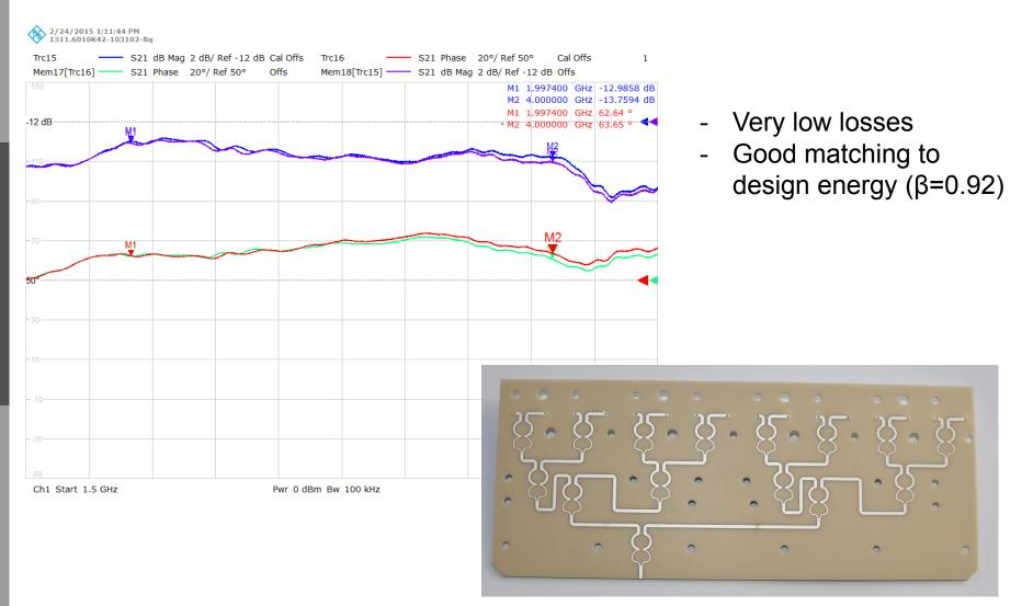
All Al<sub>2</sub>O<sub>3</sub> combiner-boards for main-system fabricated
