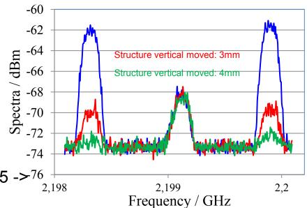
16 rings in test-tank cooled down to 30K:
