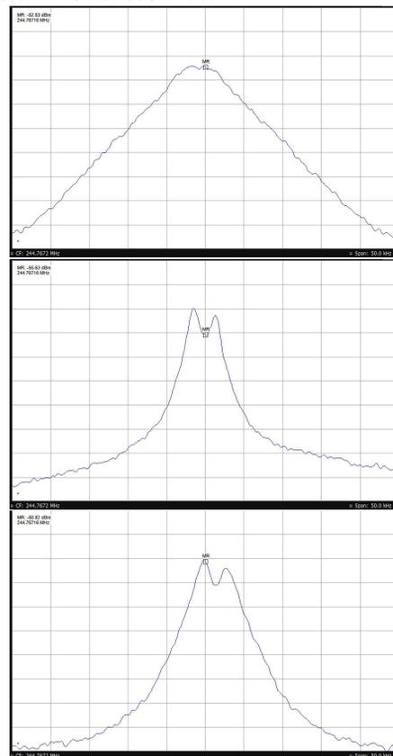
Figure 4: Schottky signal suppression (double peak structure, reduction of total integrated noise power) appearing in the momentum distribution of a beam of  $1.3 \cdot 10^9$  protons with increasing electron cooler current; top: 100 mA, middle: 250 mA, bottom: 500 mA. Frequency spectra from the resonant Schottky pickup at 245 MHz, span=50 kHz.
