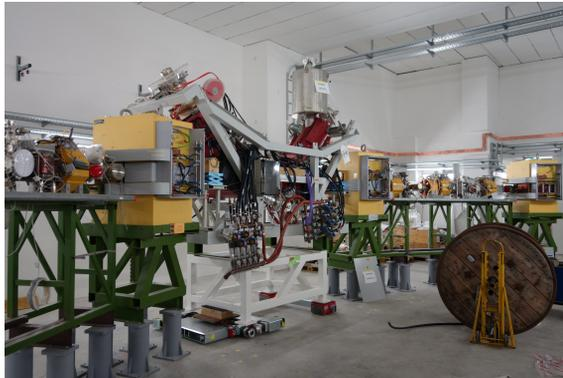
Figure 2: CRYRING cooler in the cave.
