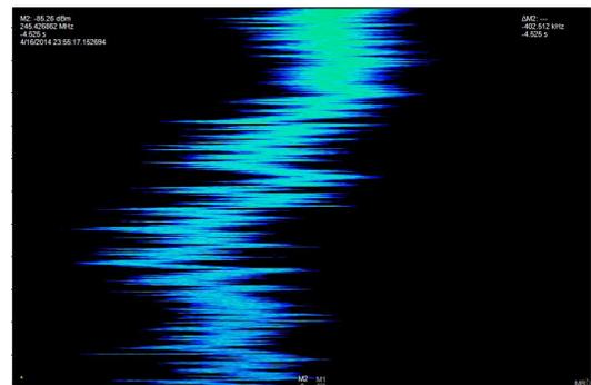
Figure 6: The instability of the electron cooler voltage observed in the longitudinal spectrum of the beam in the ESR. Frequency variation of  $\pm 5$  kHz around 245 MHz (span =20 kHz) corresponding to  $\Delta V/V = \pm 10^{-4}$  i.e.  $\pm 20$  V at 200 kV for the cooler voltage. Total recording time= 90 min.
