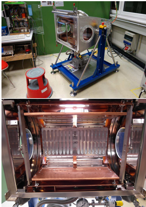
Figure 3: The chamber for lifetime tests of motor drive units and all moving components.
