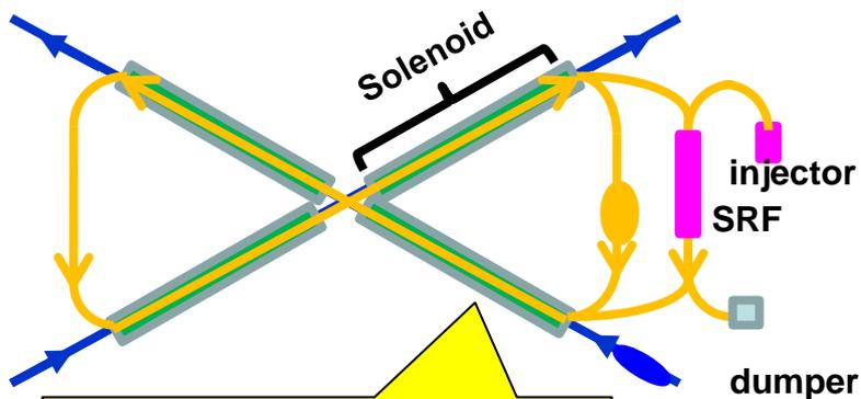
eliminating the long return path doubles the cooling rate
