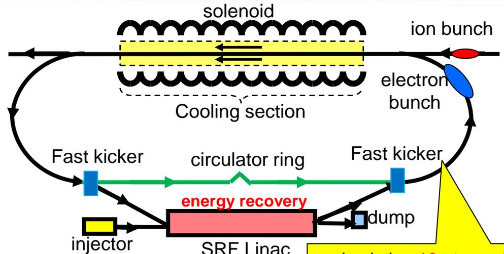
recirculating 10+ turns → reduction of current from an ERL by a same factor
