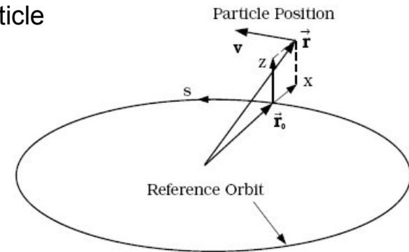
With fields  $B_x(\theta) = \frac{1}{c} E_z(\theta)$  for vertical kicker and  $B_z = -B$  the vertical dipole field
