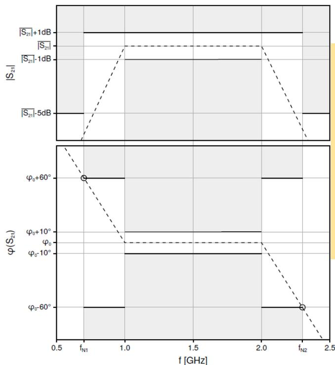
Figure 1.1: Tolerance bands for amplitude and phase of the transmission within and beyond the specified frequency range of 1...2 GHz. The gray areas are forbidden. The frequencies  $f_{N1}$  and  $f_{N2}$  are those (if any) where  $\Delta\varphi = \pm 60^\circ$ .
