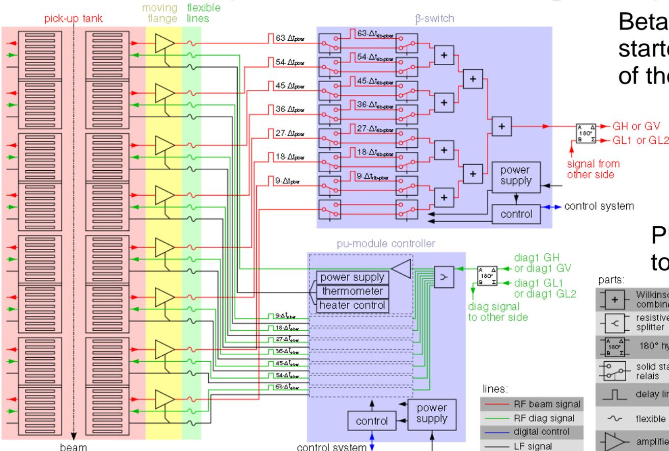
Beta switch: design ready, started in-house assembly of the small series
