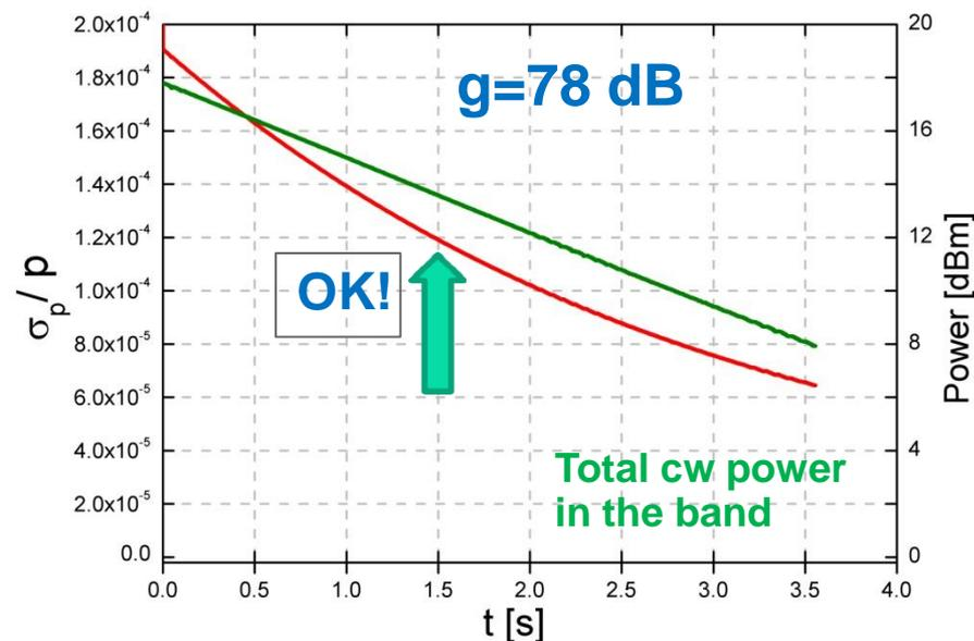
Particle noise scales with  $Q^2$ , thermal noise negligible
