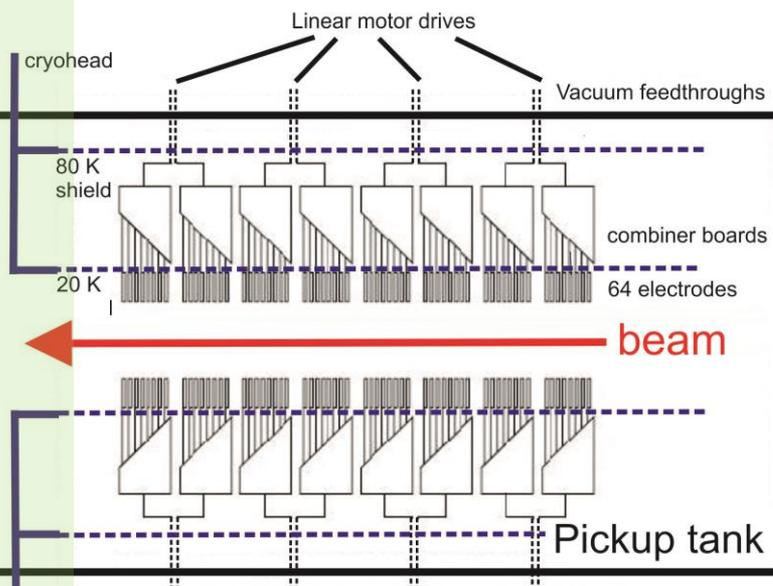
Cryo-cooling reduces considerably the thermal noise originating from the pick-up structures.
