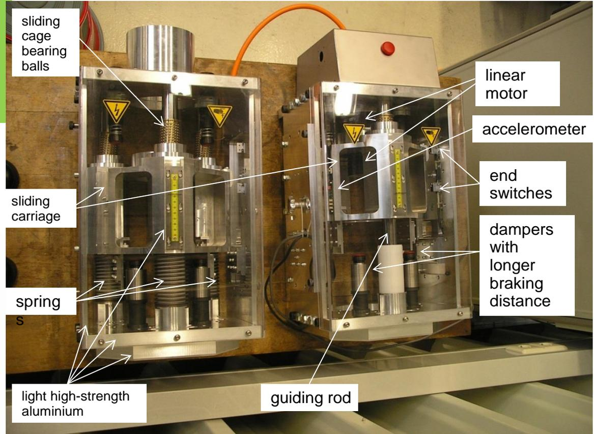
**2013: re-assembly in the tank & synchronous tests at room temperature planned**
