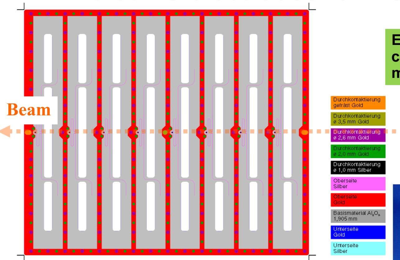
End 2012: first electrode ceramic plates delivered; metallisation pending
