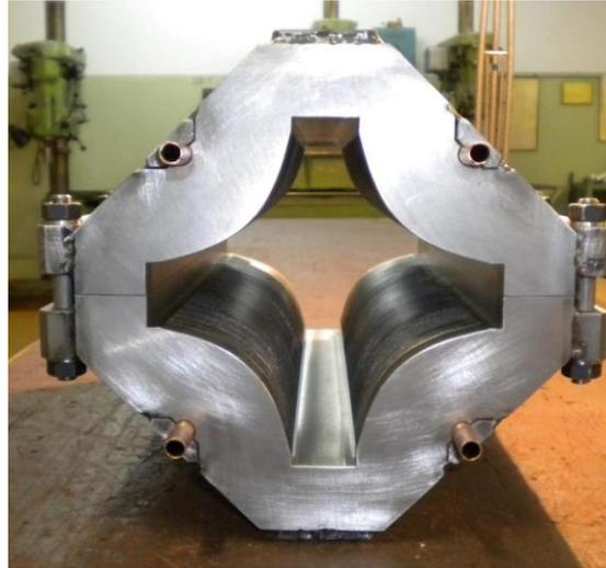
Quadrupole lense at assembly for test
