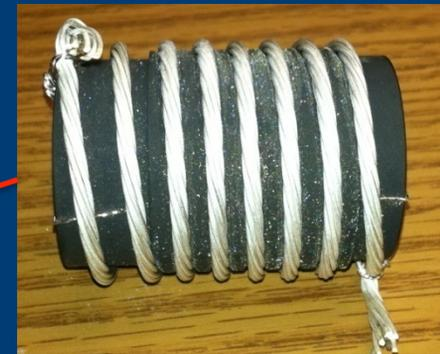
Multi-strand cable utilizing chemically compatible alloy and oxide layer to minimize cracks
