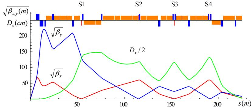
Larger chromatic function ( $W_y$ ) is corrected first with a single sextupole S1,  $W_x$  is corrected with two sextupoles S2, S4 separated by  $180^\circ$  phase advance.
