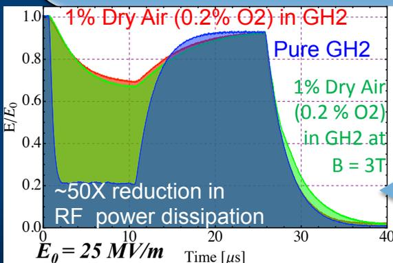
Demonstration of High Pressure RF Cavity in 3T Magnetic Field with Beam
