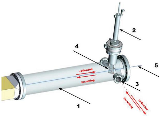
Figure 3: Laser beam input-output. (1 – vacuum chamber, 2 – push-pull manipulator, 3 – vacuum glass window, 4 – prism, 5 – proton beam axis).
