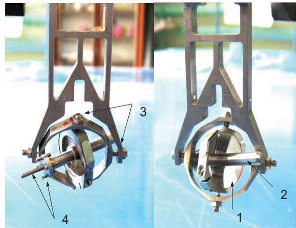
Figure 1: Compass with gimbal suspension. (1 – mirror, 2 – compass needle, 3 – jewel bearings, 4 – balancing screws).
