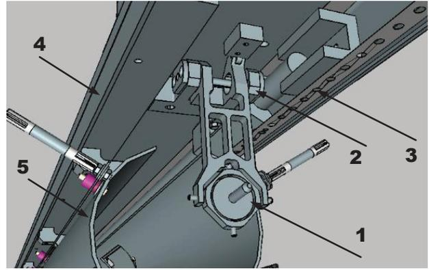
Figure 2: Compass assembly. (1 – mirror, 2 – compass driving cart, 3 – perforated tape, 4 – titanium rail, 5 – false tube).
