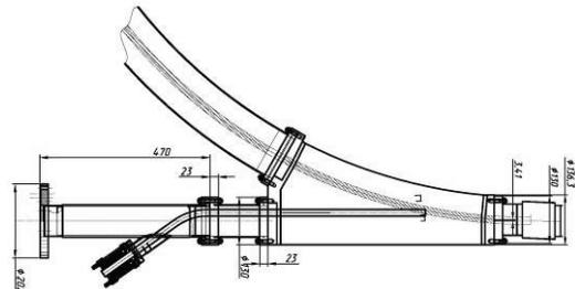
Figure 2: The circulating e<sup>+</sup> beam detector.
