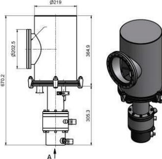
Figure 4: The cryogenic pump.
