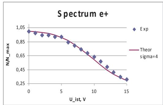
Figure 6: The spectrum of slow positrons.
