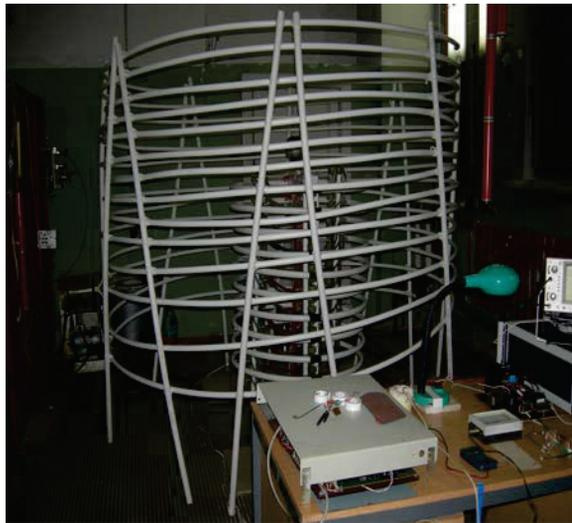
Figure 3: HV generator prototype  $U=300$  kV,  $I=1$  mA.
