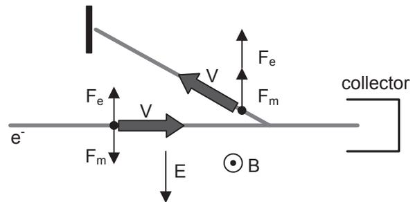
Figure 1: Principle of the collector with Wien filter work.
