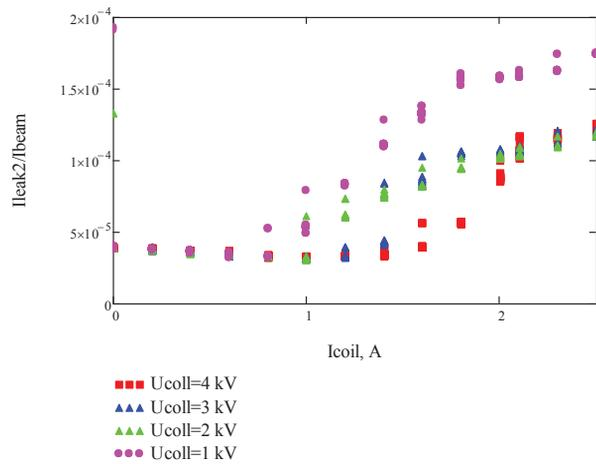
Figure 9: Dependences combined collector efficiency on current in the last coil.
