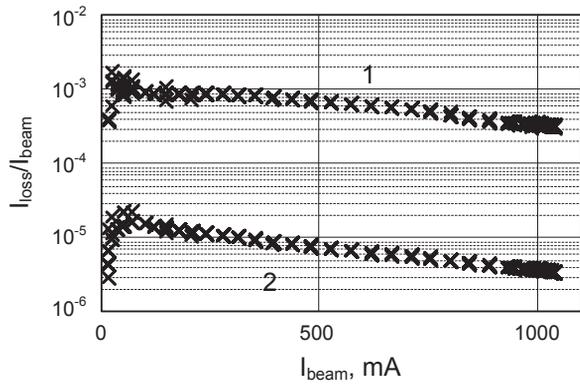
Figure 6: Dependences of the collector itself (1) and combined collector (2) efficiencies on beam current.
