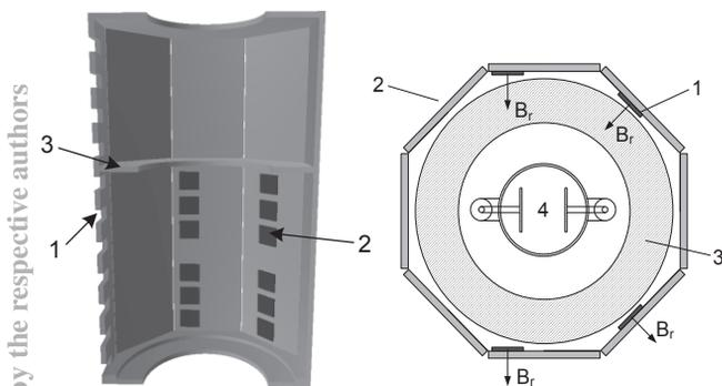
Figure 3: Left - magnetic shield with permanent magnets: 1 - holes for cooling of solenoid, 2 - permanent magnets, 3 - magnetic diaphragm. Right - top view of the Wien filter. 1 - permanent magnets, 2 - magnetic shield, 3 - solenoid for longitudinal magnetic field, 4 - electrostatic plates.
