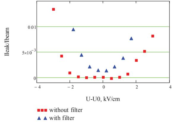
Figure 8: Dependences of leak current on voltage between plates of the Wien filter.
