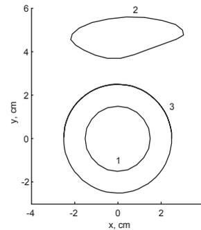
Figure 5: Shape of secondary beam after passing through the Wien filter. 1 - initial shape, 2 - shape after passing, 3 - internal size of the secondary collector.
