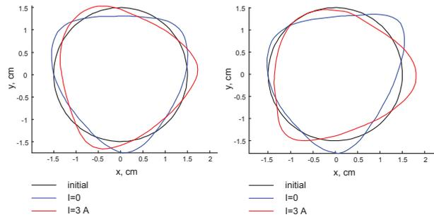
Figure 4: Main beam shape after passing the Wien filter for different values of beam current. Left - electron energy is  $E=20$  keV, right -  $E=7$  keV.
