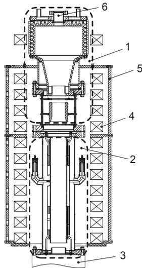
Figure 2: Sketch of the collector with Wien filter. 1 - collector itself with the suppressor and pre-collector electrodes, 2 - vacuum chamber of the Wien filter, 3 - electrostatic tube, 4 - coil for longitudinal magnetic field, 5 - magnetic shield, 6 - flange for additional vacuum pumping.
