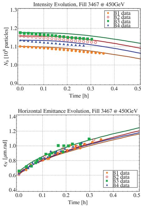
Figure 2: Intensity (top) and emittance (bottom) evolution at injection for 4 single bunches. Dots: measurement, lines: simulation.
