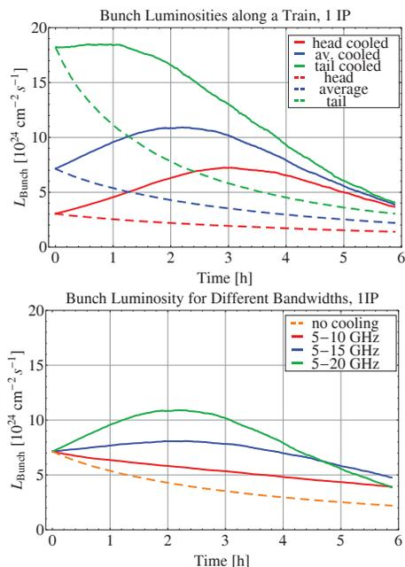
Figure 5: Top: Bunch luminosity for 3 typical bunches with and without cooling. Bottom: Average bunch from top plot for systems with different bandwidth.
