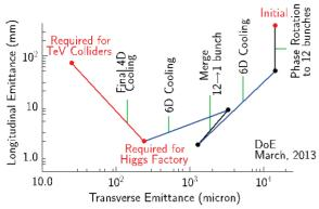
Figure 2: Emittance evolution along a 6D ionization cooling channel for a Muon Collider (MC). The entrance to the channel is the point at the upper right of the plot. The very small energy spread required for a Higgs Factory could be obtained by stopping at the bottom red point. Smaller transverse emittances, and hence higher luminosities for TeV-scale colliders, would require letting the cooling continue to the upper left red point.
