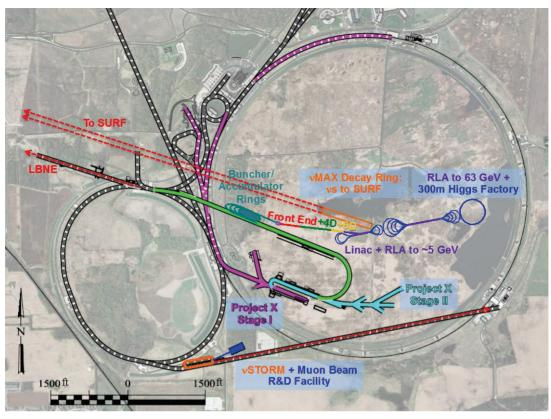
Figure 3: A staged facility, from vSTORM through the implementation of a Higgs Factory, on the Fermilab site. The second stage, implementation of the NuMAX Neutrino Factory capability, could be built on the foundation of the Project X Stage II CW Linac operating at 3 GeV proton energy.
