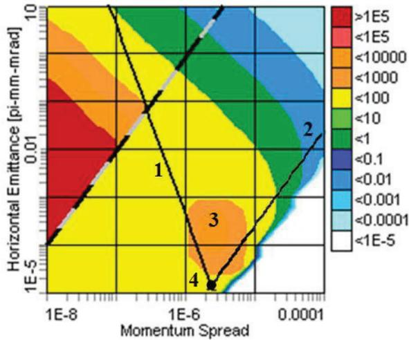
Figure 4: "3D" Dependence of IBS longitudinal heating rates (in colours) vs horizontal emittance and momentum spread of proton beam (S-LSR, 7 MeV,  $N_p = 10^3$ ); 1 – criterion (1) line; 2 – proton cooling "trajectory"; 3 – anomalous island of IBS heating of longitudinal momentum component; 4 – ordering point where the lines 1 and 2 meet.
