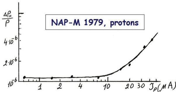
Figure 1: Proton beam momentum spread vs beam current under electron cooling in NAP-M cooler-ring [17].
