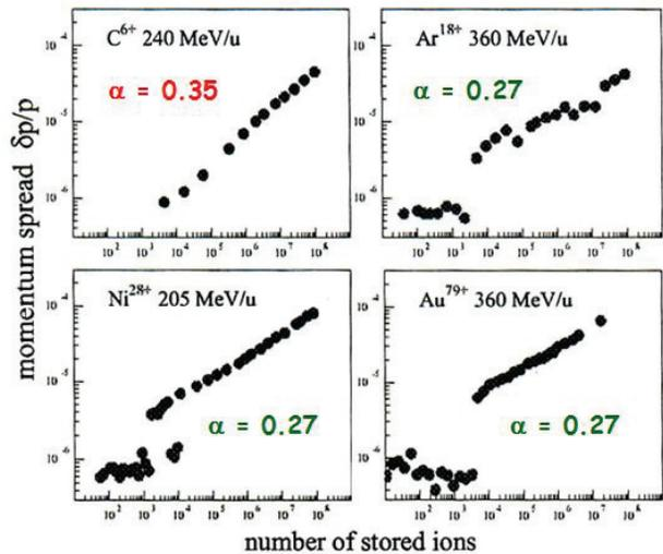
Figure 2: Ion momentum spread vs ion number under electron cooling in ESR [19].
