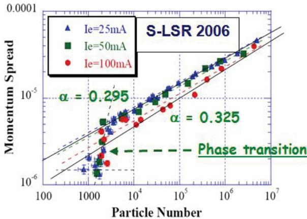
Figure 3: Proton momentum spread vs proton number under electron cooling in S-LSR [23].
