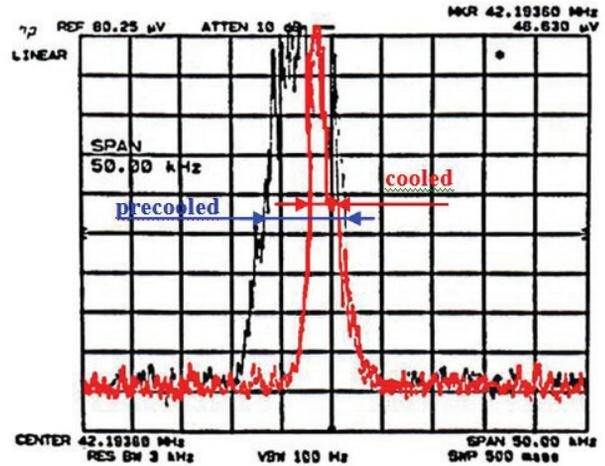
Figure 5: First Electron Cooling of Antiprotons in LEAR (CERN),  $\Delta p/p = 6 \cdot 10^{-5}$ , December 14, 1988.
