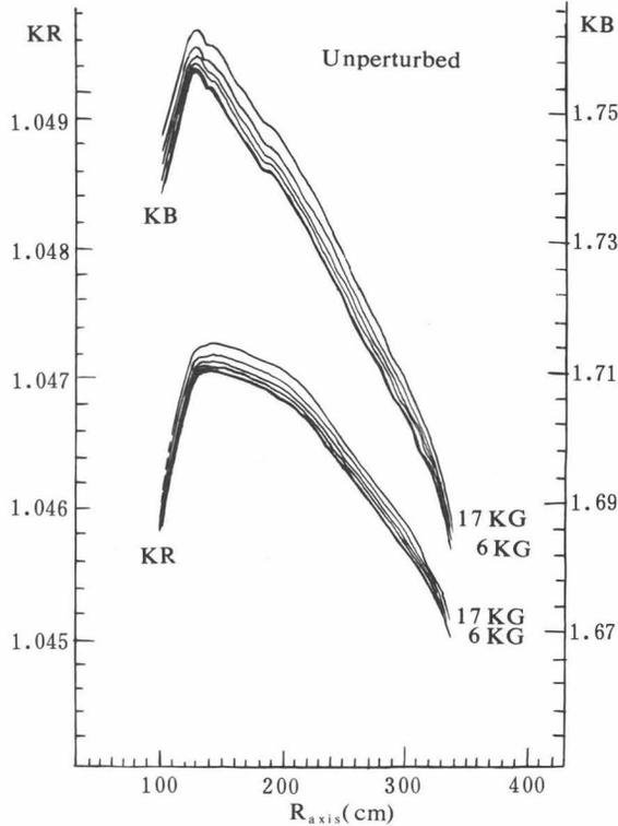
Fig.10: Kb and Kr values for the unperturbed field for 7 field levels.
