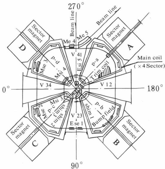
The design and construction of sector magnet were already presented in international journal<sup>[1]</sup>. Let us briefly recall its main characteristics and give the functions of the coil power supply.
