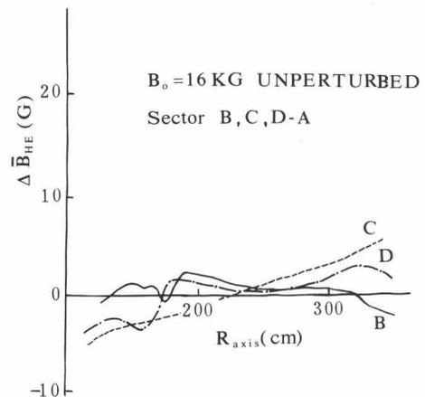
Fig.4: Comparison among the mean field differences of the sector B, C and D minus A, respectively.
