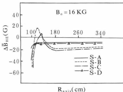
Fig.7: Effects of the injection elements for each sector after compensation by shims.
