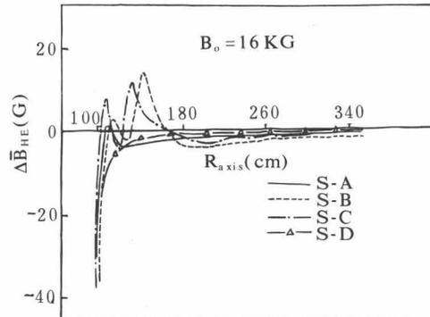
Fig.8: Remaining perturbations of the injection elements for each sector after correction by shims and correction coils.
