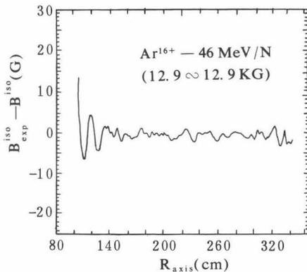
Fig.11: Deviation between the required isochronous field distribution along sector axis of  $Ar^{16+}$ -46MeV/N and measured one.
