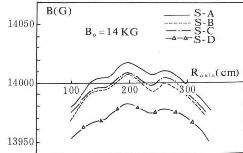
Fig.3: Unperturbed field distributions along the sector axis before balancing for 4 sectors.
