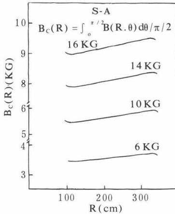
Fig.6: Mean field distributions along the radius.
